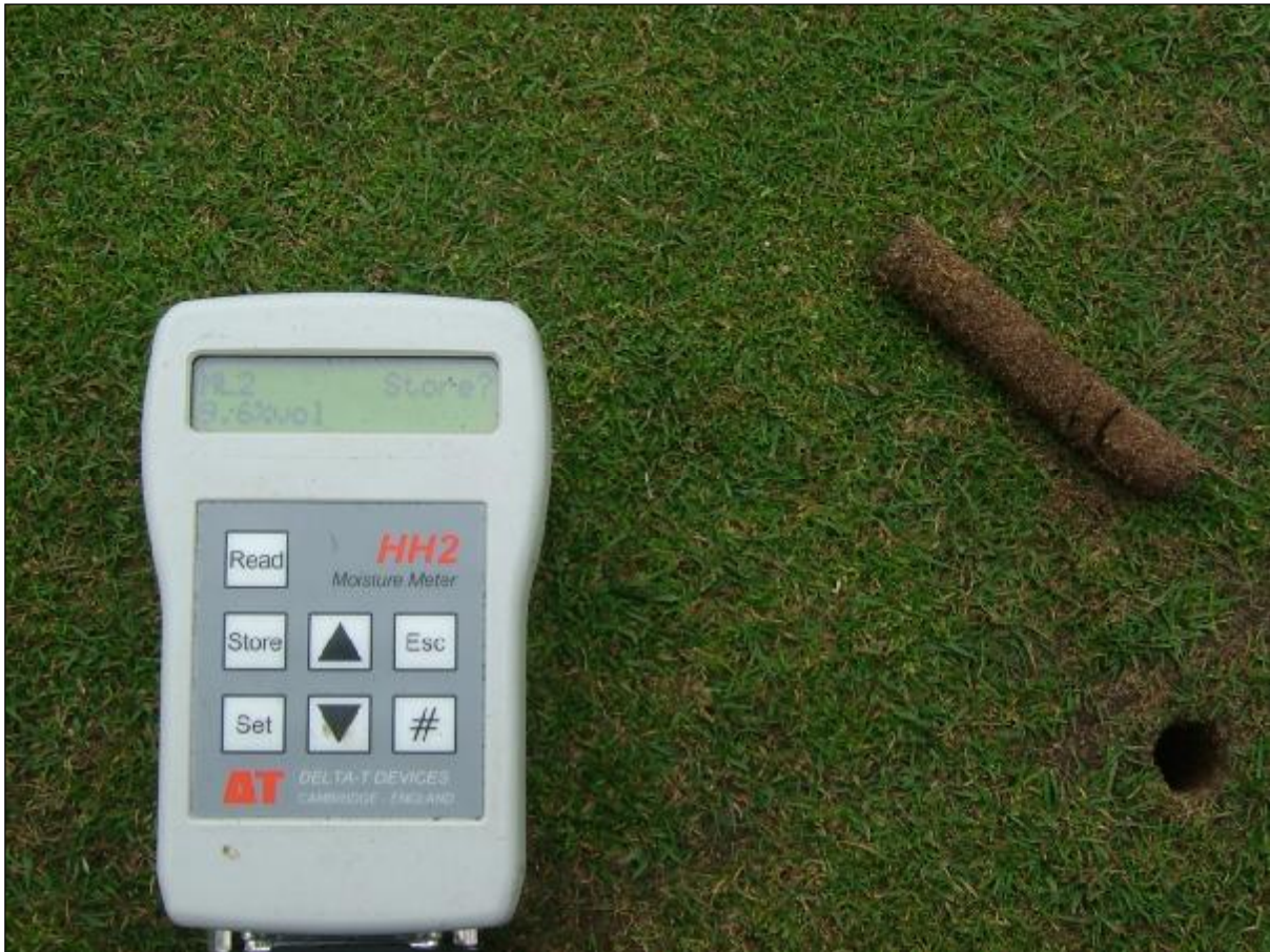
A volumetric moisture reading of 9.6% was obtained on the left hand bunker bank of the 18 th
